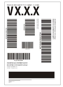
Figure 42 • FEED Self Test Label, Relative Darkness Value Zero
