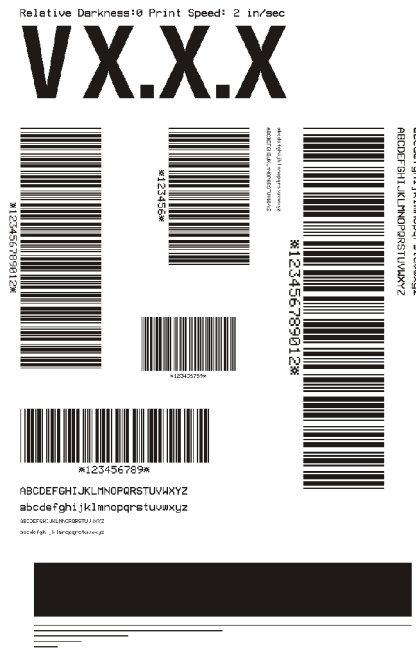
Figure 35 • FEED Self Test Label, Relative Darkness Value Zero
